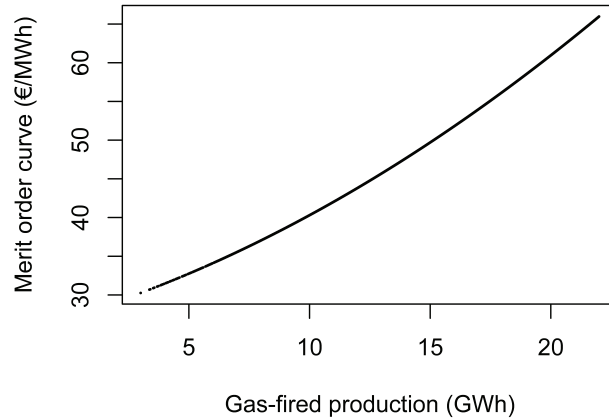
Figure 6: Estimated gas-fired merit order curve based on average gas and carbon emissions prices. Coefficients from the quadratic regression model estimated on the series for unsold electricity.
