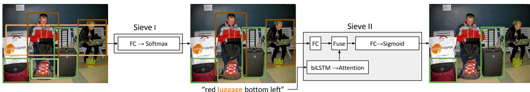
Figure 2.1: Overview of Neural Sieves. Sieve I filters object types having multiple instances. Sieve II filters objects of one category mentioned in referring expression. Objects of the same category have the same color frames. Best seen in color.
