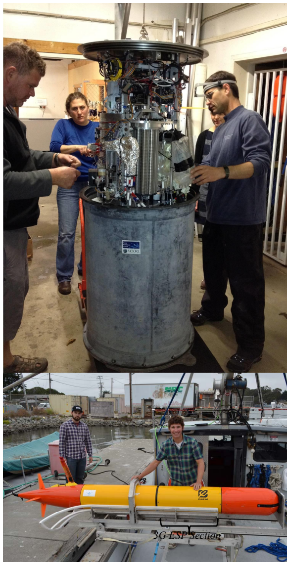
Fig. 2: Size comparison of two ecogenomic sensors. Top: 2 nd Generation ESP, loaded with reagent bags and media filters, is being lowered into a 215L pressure housing for deployment on a mooring. Bottom: Long Range AUV Makai with 3G-ESP assembled for deployment. The marked section of the AUV contains the G3-ESP instrument in a 40L space.
