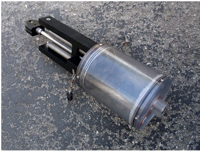
Fig. 3 A single Gulper water sampler with 1.85 L capacity.
