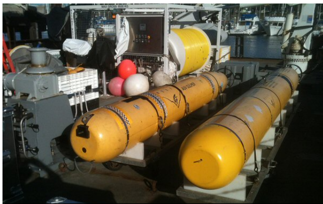
Fig. 1 CTD/Gulper AUV (left) and Seafloor Mapping AUV (D. Allan B.) on the deck of MBARI's R/V Rachel Carson.
