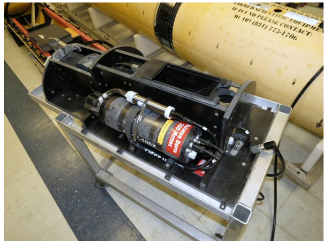
Fig. 2 CTD/Gulper AUV Science Payload (removed from nose of vehicle.)
