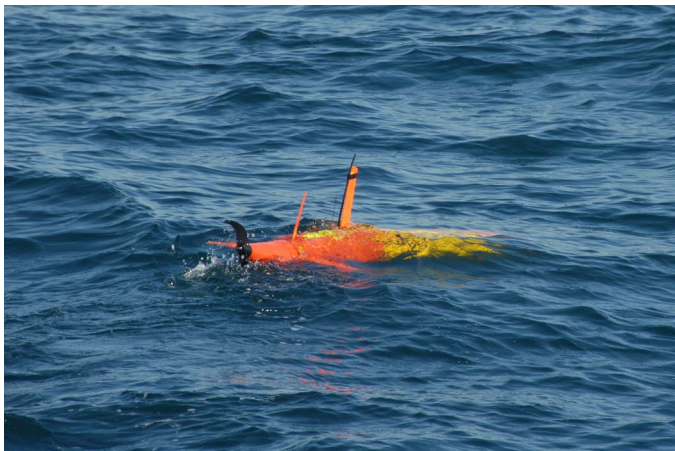
Fig. 1. The Tethys AUV deployed in Monterey Bay. The orange tail section of the vehicle is the propulsion and control section, which also includes antennae for Iridium and Argos satellites, GPS, and line-of-sight radio-frequency communications. The yellow center section is the main pressure vessel housing vehicle electronics and batteries. The orange head section (submerged) is a wet volume housing a suite of science sensors.
