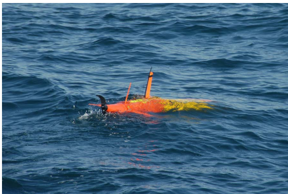
Fig. 4. The Tethys AUV deployed in Monterey Bay. The orange tail section of the vehicle is the propulsion and control section, which also includes antennae for Iridium and Argos satellites, GPS, and line-of-sight radio-frequency communications. The yellow center section is the main pressure vessel housing vehicle electronics and batteries. The orange head section (submerged) is a wet volume housing a suite of science sensors.
