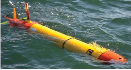
Fig. 1. The Makai long range AUV which is equipped with a 3G-ESP.
