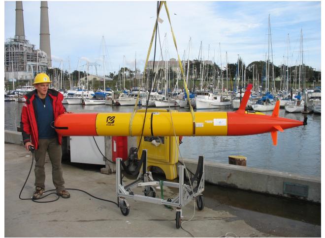
Fig. 1. MBARI Long Range Autonomous Underwater Vehicle (LRAUV).
