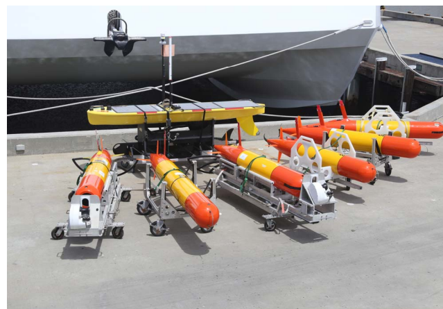
Figure 1: Five LRAUVs, one with 3G-ESP payload, two on launch and recovery systems (LARS) and a Wave Glider SV3
