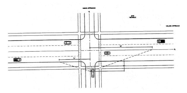
Figure 9-2. Minimum Required Site Triangle
