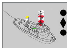
Vessel engaged in towing operation which severely restricts towing vessel and her tow in their ability to deviate from their course Length of tow does not exceed 200 meters; towing vessel less than 50 meters in length
