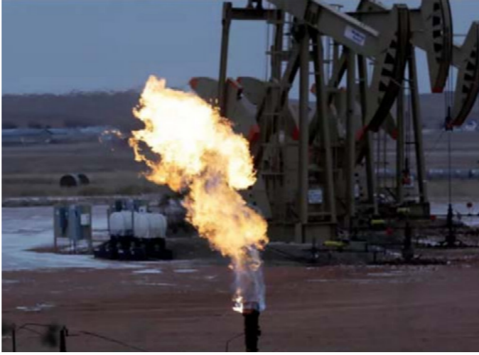
A flare stack at a wellhead. Source: South Coast Air Quality Management District.
