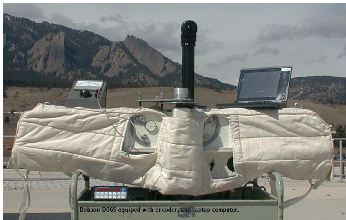
A Dobson spectrophotometer. Source: https://gml.noaa.gov/ozwv/dobson/
