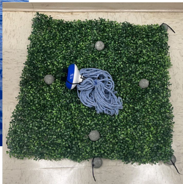
Left: A drifter with a GPS tracker is deployed near a Sargassum mat. Right: Artificial Sargassum with a GPS-equipped drifter attached. Source: NOAA AOML.
