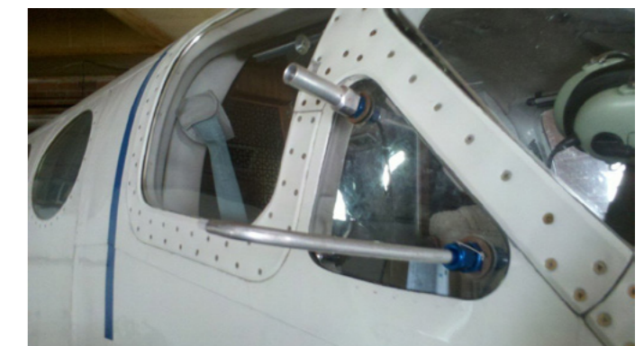
Clockwise from top left: Ambient surface air sampling unit (source: CARB), balloon launch of an ozonesonde (source: NOAA GML), sampling ports on aircraft (source: NOAA GML).
