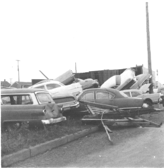
Figure 28. Cars stacked up at Harbor Motors, Second and L Street, Crescent City. Note that the lighter trunk end of the cars floated up onto the heavier motor ends. (Used by permission, Wallace Griffin, Crescent City Printing Co.)
