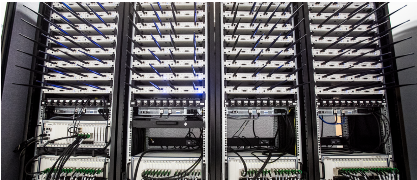
FIGURE 3 University of Bristol and Lund University implemented the world's first 128-antenna, real time massive MIMO testbed using a combination of NI commercial-off-the-shelf hardware paired with LabVIEW software. Visit ni.com/Massive-MIMO to learn more about the solution.
