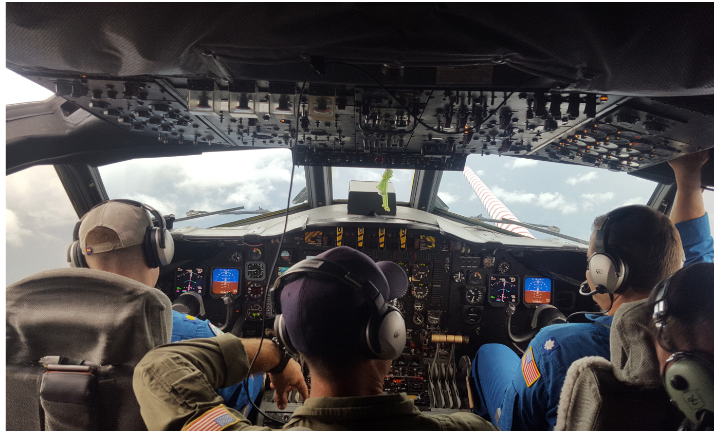
The flight deck of NOAA Lockheed WP-3D Orion Hurricane Hunter during a flight into Hurricane Harvey.
