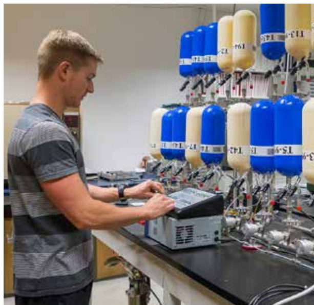
Eric Moglia, of NOAA's Cooperative Institute for Research in Environmental Sciences, pumps air from sampling flasks to test them for leaks before preparing them for shipment to some 80 sites around the world. Photo Credit: Willfred von Dauster, NOAA
