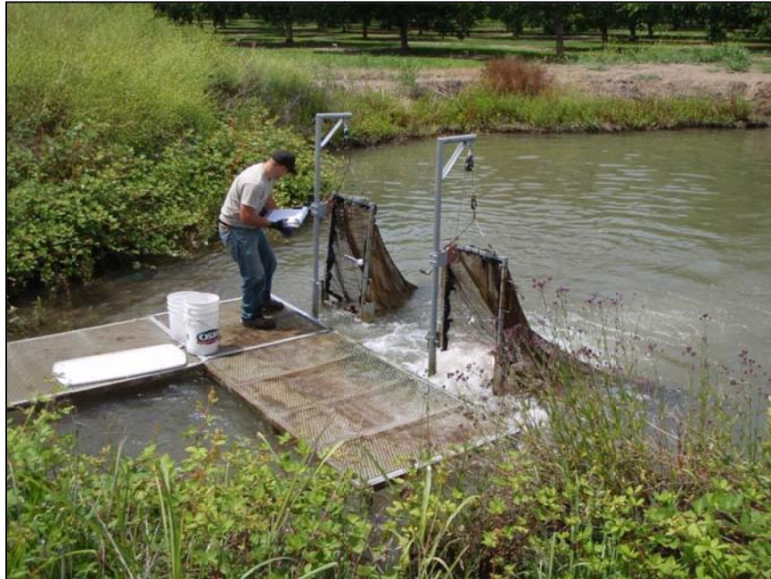
Figure 2. Fyke apparatus and nets used to sample for fish entrapment at the Sycamore canal.
