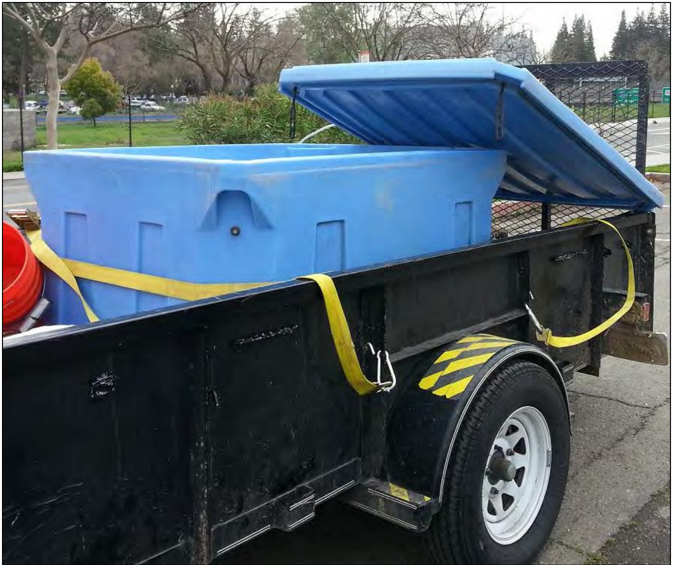
Figure 2-17 Insulated Transport Tank
