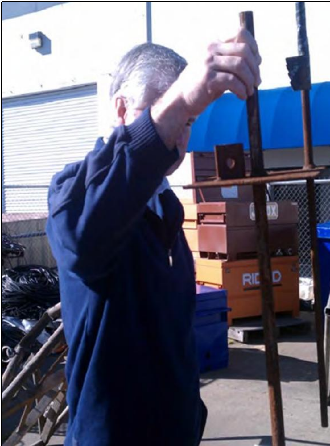
Figure 2-9 Typical “Pound-In” Bottom-Mount
