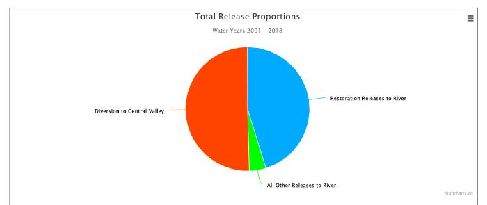
Prior to the 2000 Record of Decision (ROD), diversion to the Central Valley averaged 74%. Under the ROD exports were expected to drop to 52%. This pie-chart shows the actual proportions according to flow measurements beginning from water year 2001. [Reference: USDI 2000, page 20.]
