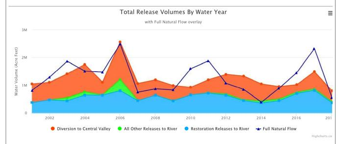
This graph provides information on water releases per water year (colored bands) relative to the reservoir inflow (dark blue line, Full Natural Flow). Total releases need not match the inflows within each year because the reservoir allows storage or usage of water. Periods where the dark blue line rises above the colored bands indicate net increases in reservoir storage while periods where the dark blue line falls below the top of the colored bands indicate net reduction of water storage.
