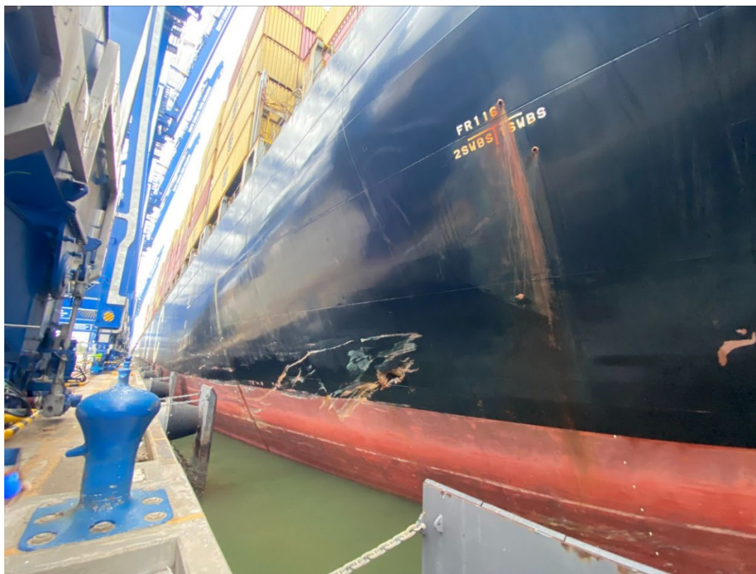
Figure 8. Damage to the MSC Rita 's starboard hull. (Source: Coast Guard)
