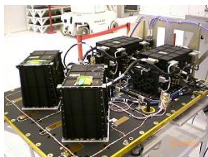
Figure 3 : Jason-3 Poseidon-3 Instrument
