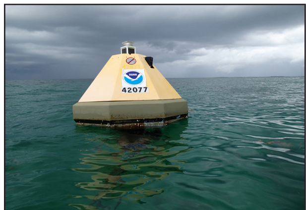
An ocean acidification buoy at Cheeca Rocks, an inshore patch reef within the Florida Keys National Marine Sanctuary. Credit: NOAA
