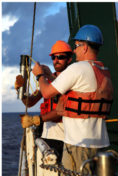
Fig. 13. Cornel de Ronde (right) and Trevor Goodman attach the MAPR to the dredge cable.
