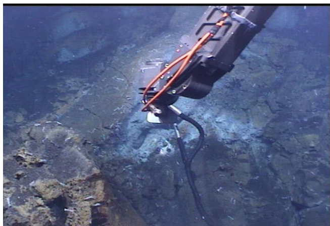
(left) Dive 414 2009/05/07 11:03:42 Shrimp City beginning to sample. Sampled 14.9degC water here with in-situ pH of 5.63. Filtered bag 19, unfiltered bag 23, sterivex 14. (right) Dive-414 End of sampling at Shrimp City.
