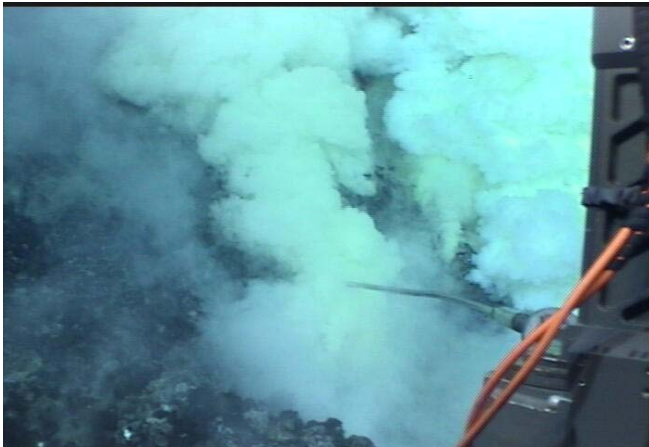
(left) Dive 418 2009/05/11 14:42 Conditions at start of filtered piston #5 at Afi vent. (right) Dive 418 14:43:47 Still taking HFS filtered piston 5 at Afi. Note tephra produced at vent to the right.
