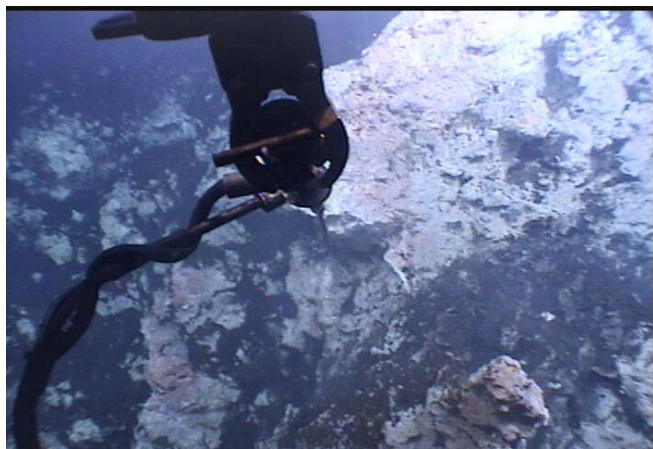
(left) Dive 417 2009/05/10 10:20:24 Measured average pH of 4.22 at 17.4°C, H 2 S voltage 0.281 at start of sampling, but the manifold was not flushing well. Later at this same site, got good flow, with pH of 2.599, H 2 S voltage 0.393, and average 28.0°C. (right) Dive 417 2009/05/10 10:31:13 Down-looking view of HFS setup at Epsilon site, near Red Rock Ridge. Collected bag 22, 23 (failed), 19, sterivex 14. No gas-tight here.
