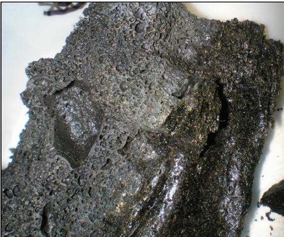
Close-up of Puipui sample J2-415-R07 showing abundant vesicles and a fresh glass rind.
