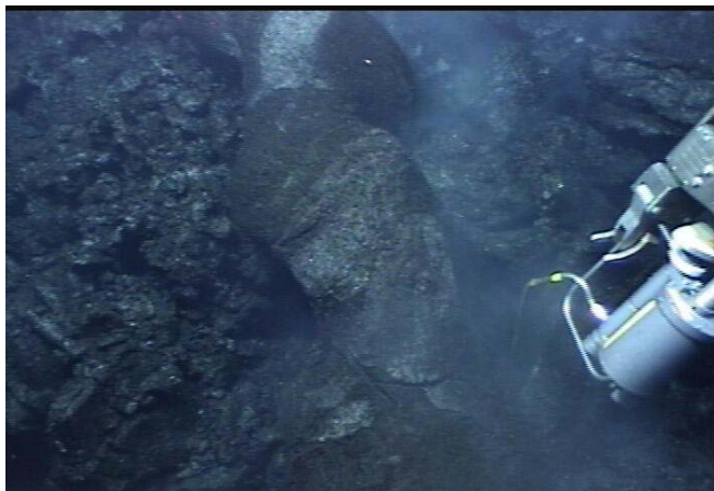
(left) Dive 420 21:31 Taking yellow major #6C in cloudy fluid emanating from recently formed pillow mound. This is 4 meters below the flaming volcanic vent.
