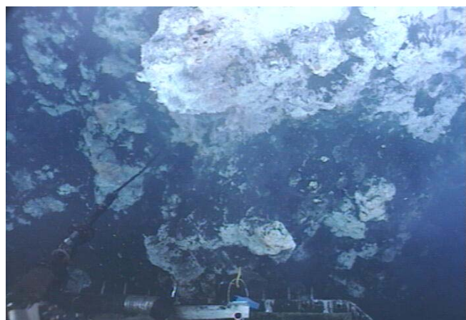
(left) Dive 417 2009/05/10 10:20:24 Measured average pH of 4.22 at 17.4°C, H 2 S voltage 0.281 at start of sampling, but the manifold was not flushing well. Later at this same site, got good flow, with pH of 2.599, H 2 S voltage 0.393, and average 28.0°C. (right) Dive 417 2009/05/10 10:31:13 Down-looking view of HFS setup at Epsilon site, near Red Rock Ridge. Collected bag 22, 23 (failed), 19, sterivex 14. No gas-tight here.
