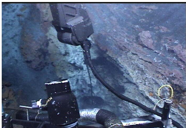
(left) Dive 417 2009/05/10 07:57:28 Another view of the Luo sampling site, 1278m, heading 102. Temp up to 22.7°C and in-situ pH of 5.1. Took 4 samples, unfilt bag 21, filt piston 5, sterivex 15 and GFF 20. (right) Dive 417 2009/05/10 10:04:47 Wide view of “Epsilon” site (z=1187, heading 141) that is near Red Rock Ridge (z=1182, heading 41).
