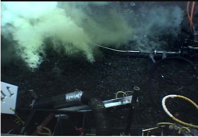
(left) Dive 418 2009/05/11 12:44:39 Hades vent during unfiltered piston 4. Venting has remained stable for 15 minutes. (right) Dive 418 12:49 Hades vent sampling filtered bag 18. Conditions still stable. Diffuse white smoke venting in the foreground has decreased. Temperature measurements beneath the surface were 4°C in foreground, 114°C under the white smoke, and 162°C under the point where we sampled.
