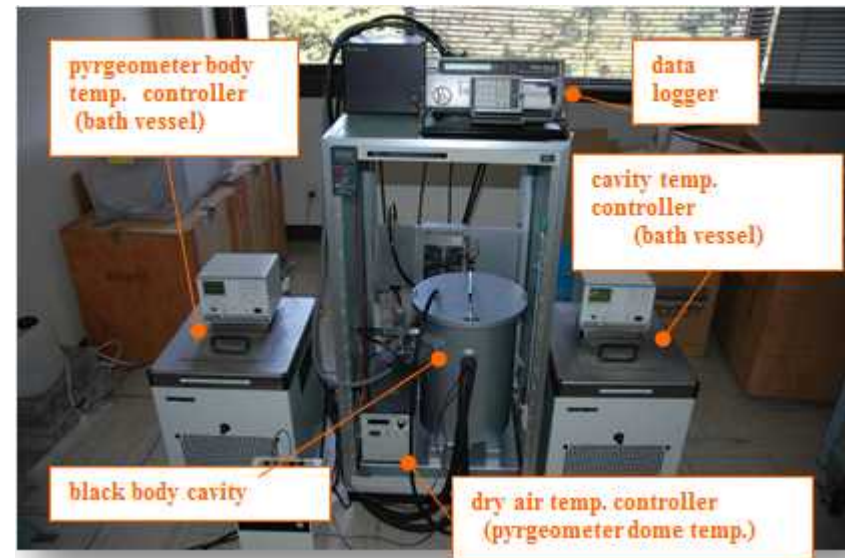
Temperature dependency test in the BB cavity
