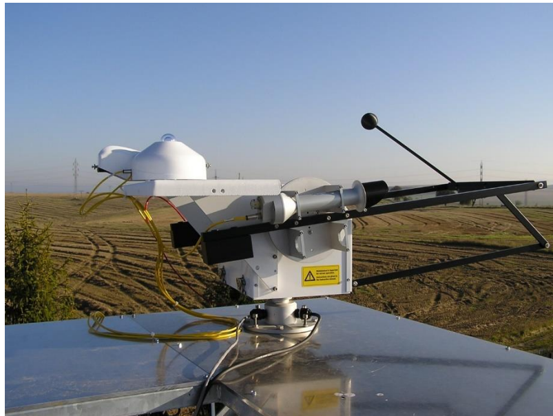
Ventilated shaded pyranometer on the solar tracker
