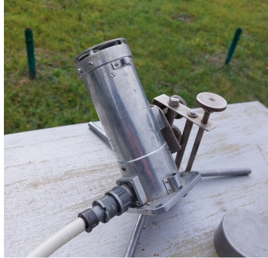
Two M-59 pyrhelimeters (Angstrom type) № 14 & № 15 (designed by MGO in 1970's)
