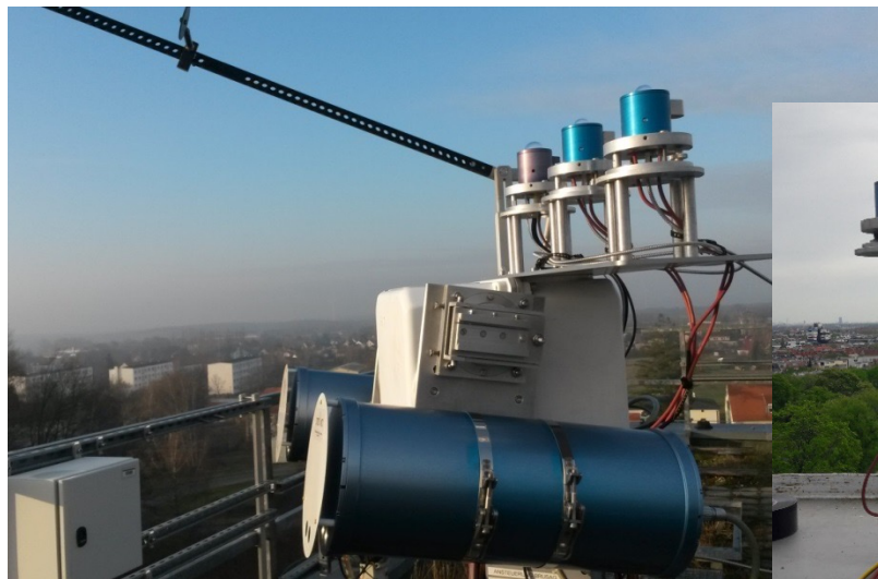
Precision spectrometer (PSR, 300-1020 nm)
