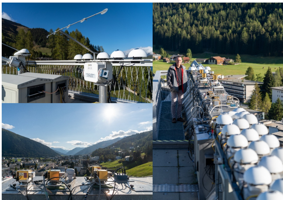
Figure 1. Pictures of the measurement platform of WRC-IRS on top of the PMOD/WRC. Left upper figure: World Infrared Standard Group (WISG), left bottom: the IRIS, right : Pyrgeometers in the foreground, IRIS and ACP in the background.
