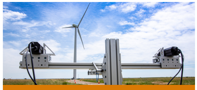
PNNL's ThermalTracker-3D technology is a stereo-vision solution for evaluating flight tracks of birds and bats around wind turbines. (Photo by Werner Stocum, NREL)
