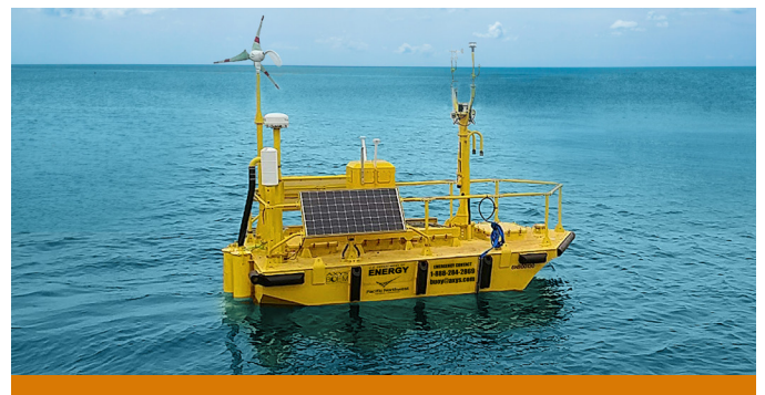
Department of Energy lidar buoy deployed off Morro Bay, California. (Photo by AXYS Technologies and PNNL)
