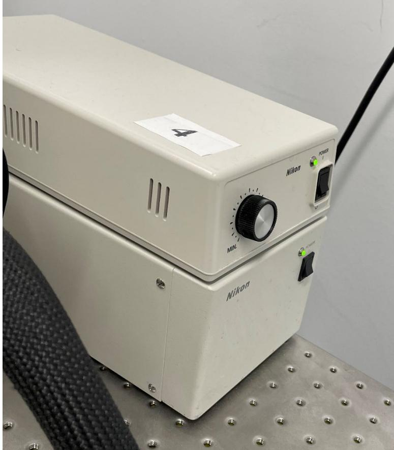
5. Turn on the power of the microscope (right bottom side of microscope).
