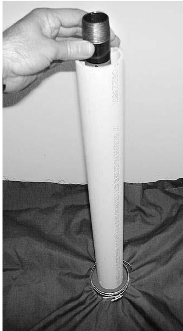
Figure A3.7 - Drop Tester just before making a test drop. Note that the guide tube is centered on the clamped fabric, and the drop probe is being used as a plumb bob to make the guide tube vertical.
