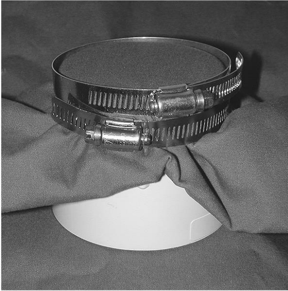
Figure A3.6 - Fabric clamped onto flange with two hose clamps. Notice that the second one will protrude a bit above the level of the fabric with thicker fabrics, but it should still be tight if you push everything down enough.
