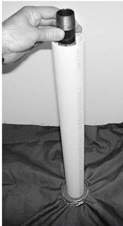
Figure A3.1 - Drop tester (pipe end sticking out of white guide tube) ready to use on some fabric clamped onto the 3" flange.
