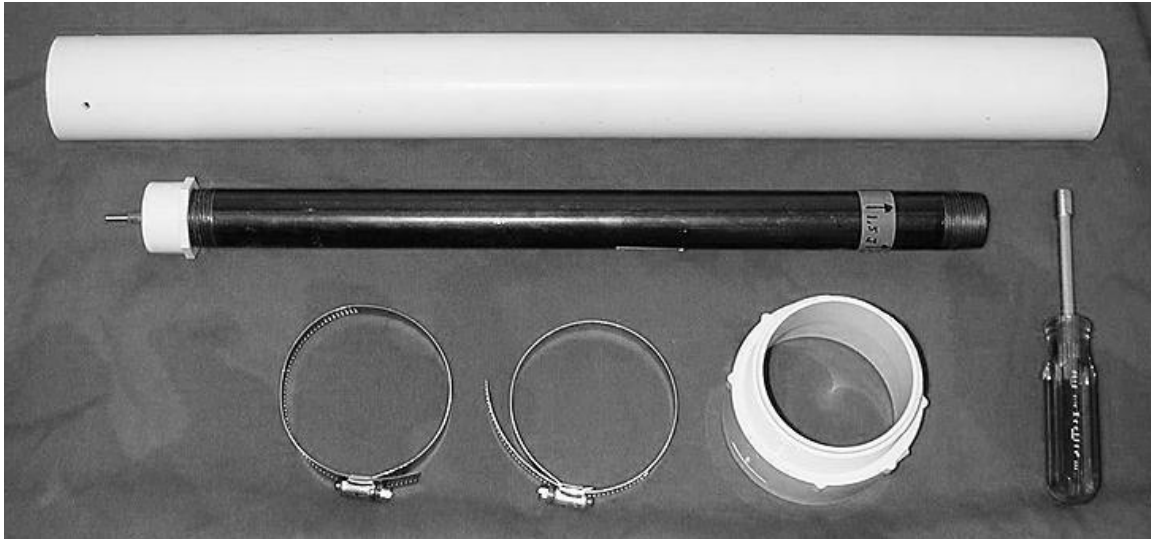
Figure A3.5 - Parts needed for SCA Standard Drop Tester for fencing armor.
