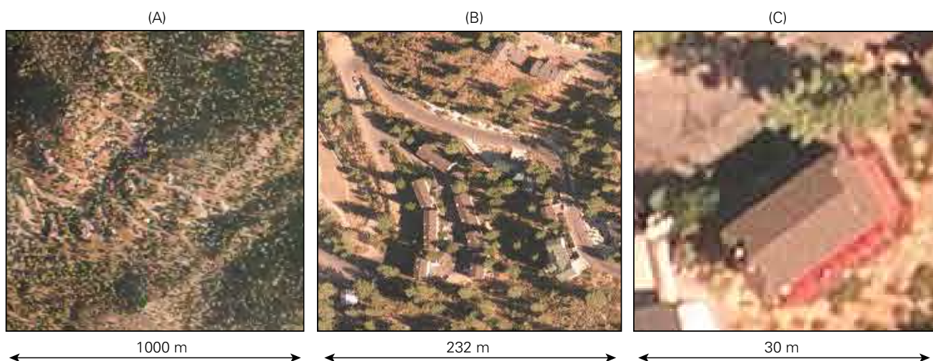
Figure 9.6—Mixed vegetation or land cover types that can result from different spatial resolutions, including: (A) 1000 m, (B) 232 m, and (C) 30 m grid cell widths. Products delivered at these resolutions would only provide one value for each unit area above, which typically decrease in diversity from left to right depending on the patch size of the vegetation.
