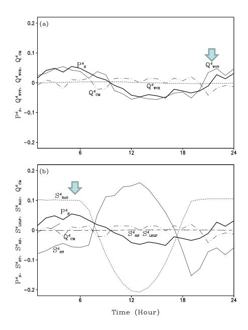
Diurnal anomalies of surface rainfall equations from equilibrium model simulations imposed with zero large-scale vertical velocity and 29°C of sea surface temperature
