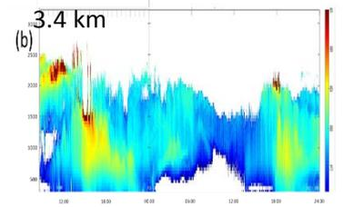
Coherent Doppler Lidar Attenuated Backscatter
