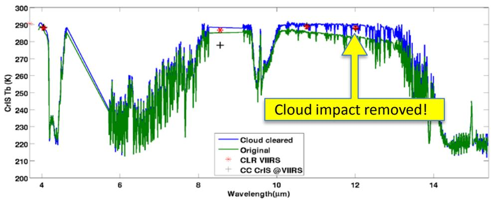
Collocated high resolution imager data from VIIRS provide cloud mask for CrIS to do clear detection. With the cloudy information, partially cloudy CrIS FOVs can be cloud-cleared successfully.
