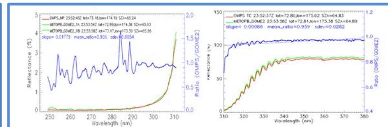
Figure 1: SNO Validation in reflectance comparisons between OMPS NP and GOME-2 Band 1A and between OMPS NM/TC and GOME-2 Band 2B.
