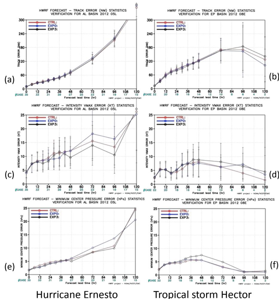
Figure 1 Forecast performance verification for Hurricane Ernesto and Tropical storm Hector. (a) and (b) are track errors, (c) and (d) for intensity error; (e) and (f) for minimum center pressure error. Red assimilates infrared and cloud top water vapor AMVs very 6 hours from heritage algorithm,; blue assimilates the same type of winds as red but from the GOES-R algorithm with hourly frequency and black includes hourly and high temporal AMVs for all wind types from GOES-R algorithm.
