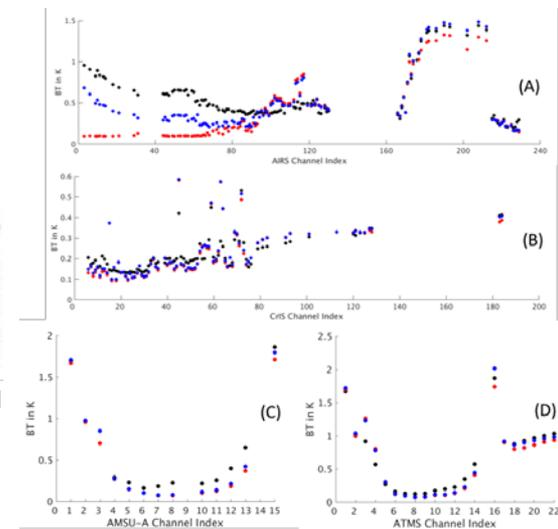
Figure 3 Standard deviation for innovation of BT in K for (A) AIRS, (B) CrIS (C) NOAA-18 AMSU-A and (D) ATMS. Real world in black, before variance calibration in red and after 1 iteration of variance calibration in blue.
