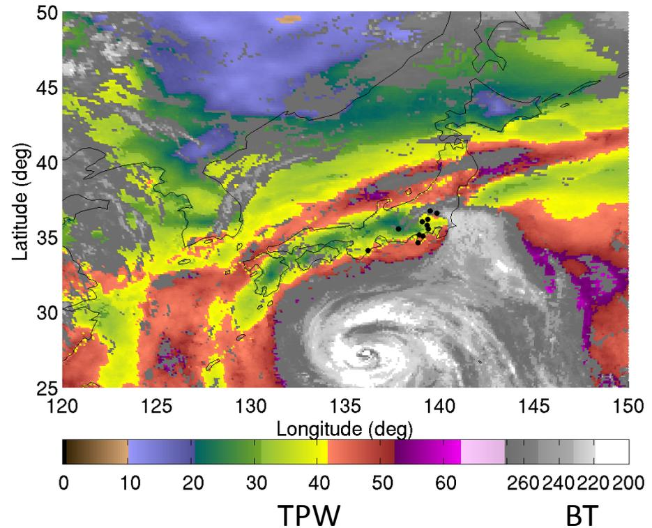
TPW (Total Precipitable Water) over clear skies with 11  $\mu$ m brightness temperature in gray valid at 00 UTC July 15, 2015. Black dots indicate the selected 11 ISD locations.
