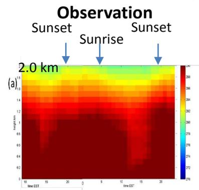
Microwave Radiometer Temperature Profile
