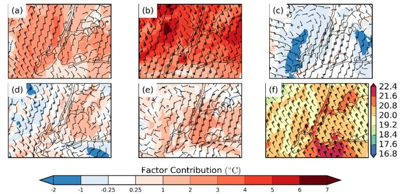
Factor contributions for (a) impervious surface, (b) heatwave only, (c) impervious surface/urban fluxes, (d) impervious fluxes/heatwave, and (e) all factor interaction. Panel (f) is the baseline field.
