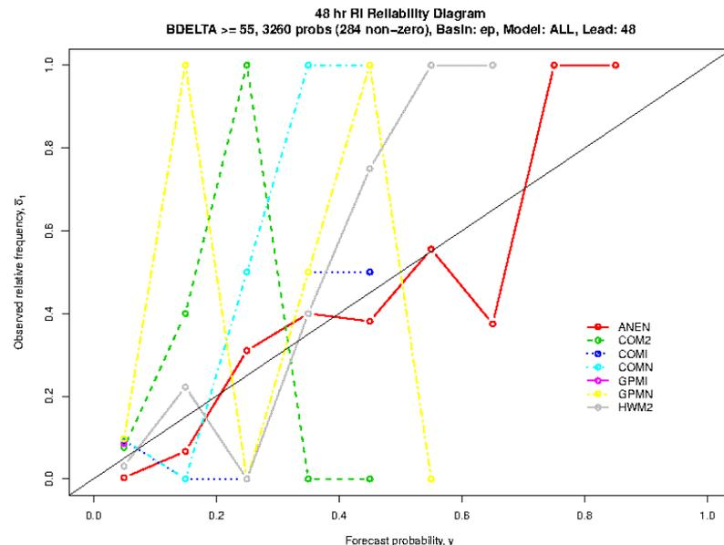
Reliability diagram for 0-48 h rapid intensification probability (55 kt intensity change threshold) for the 2014-2015 eastern Pacific hurricane seasons. Included are HFIP Ensemble Tiger Team models, including the AnEn, COAMPS ensembles, GFDL ensembles, and HWRF ensemble (Image Credit: Ryan Torn and DTC)
