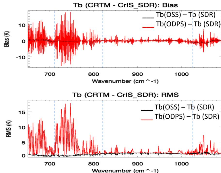
**Figure above:** Difference of CRTM-OSS (black curve) and CRTM-ODPS (red curve) simulated brightness temperatures against CrIS SDR Band1 observations under clear sky condition and with 2 absorber gases (WV, O3) over ocean for 10770 profiles.
