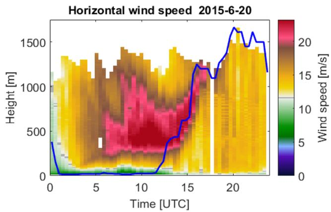
Jet wind speeds with mixing layer height plotted as blue line
