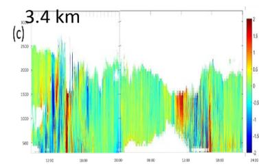
Coherent Doppler Lidar Vertical Velocity
