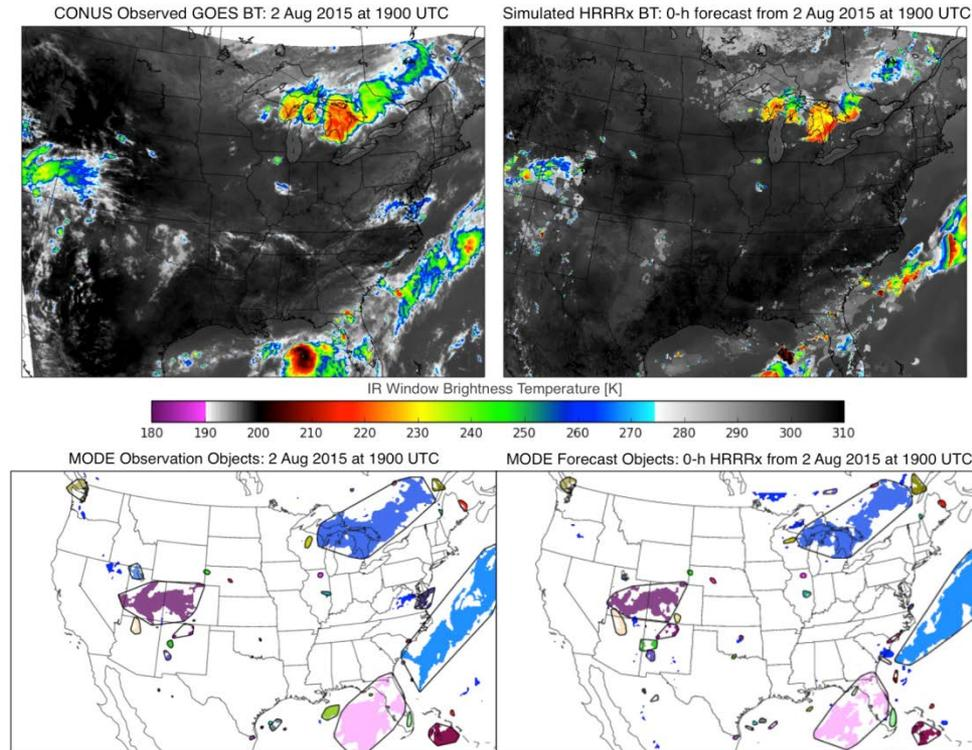
GOES (top-left) and HRRR (top-right) BTs and objects (lower) generated by the Method for Object-Based Diagnostic Evaluation.
