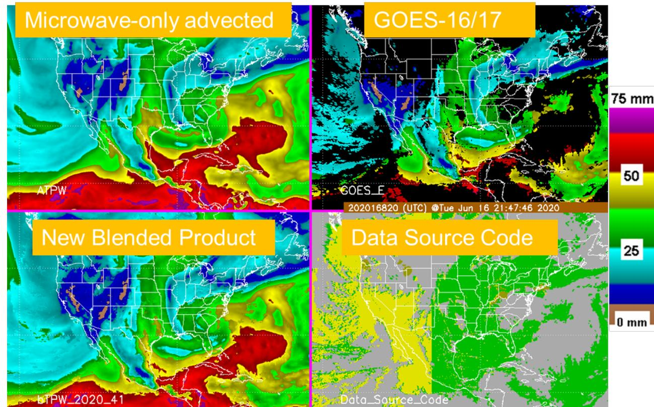
Using GOES-16/17, advected microwave data and GPS to improve performance of the blended Total Precipitable Water (TPW) product
