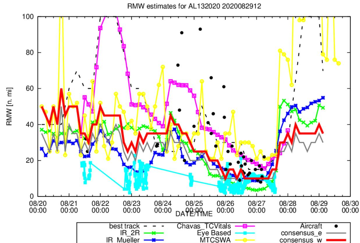
Caption: Example of Radius of maximum wind estimates for Hurricane Laura based on five methods (IR\_2d, Mueller, Chavas, Eye, MTCSWA). two consensus methods (equal, weighted) and aircraft-based observations (black dots)
