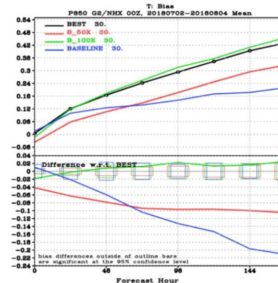
Northern hemisphere forecast bias for GFS 850 hPa temperature. (Left) Detector Noise (Right) Detector bias. The outline bars represent the 95% confidence level.
