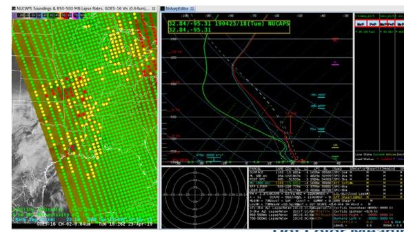
**Gridded NUCAPS** provides temperature, moisture, and stability indices (CAPE, lapse rate, etc.) at specific pressure level(s).
