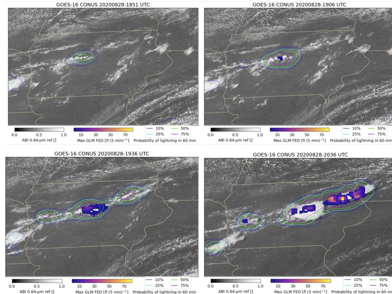
A sequence of images with probability of lightning (contours), GOES 0.64- $\mu\text{m}$  reflectance (shaded grayscale), and 5-min maximum GLM flash-extent density (shaded color) for a developing cold front in Iowa.
