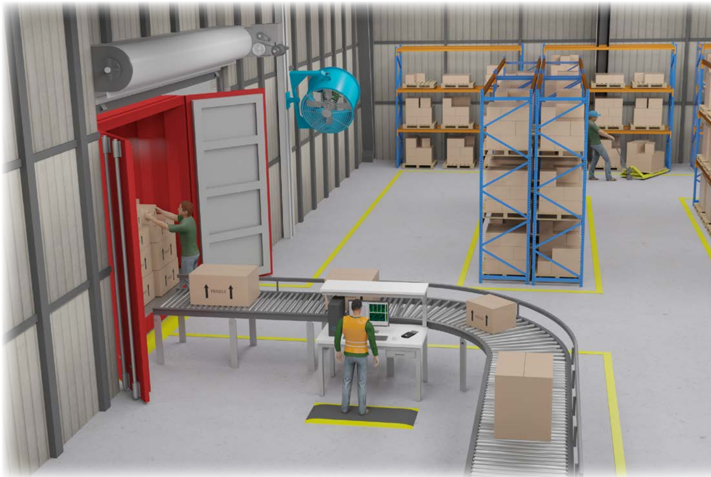
Shipping Department Exhaust Application
