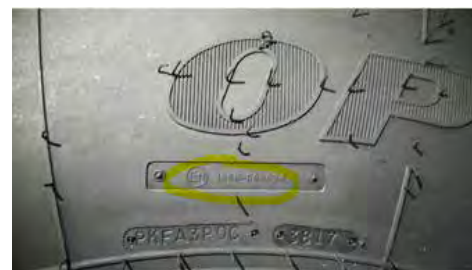
Example of the ECE Marking Note: The location of the marking on the tire may vary
