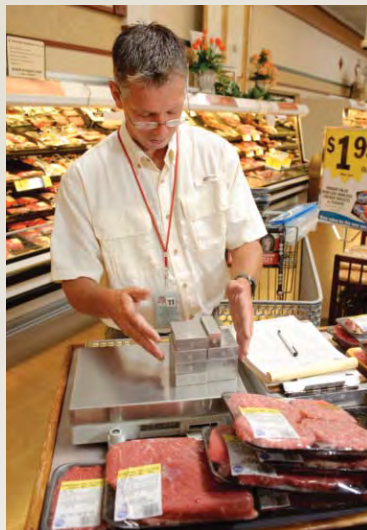
Inspectors also check their own scales for accuracy before weighing items.
