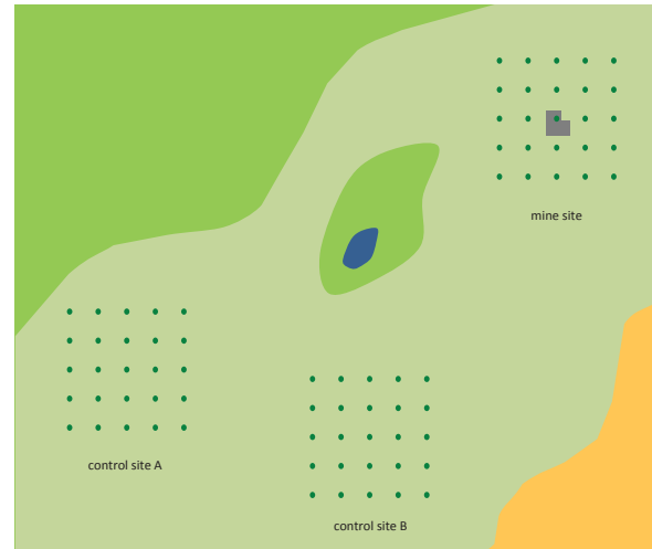
Figure.2 diagram of sampling sites for monitoring vegetation change in the vicinity of a mine site and at control sites using a before-after control-impact (BACI) design (Smith 2002).
