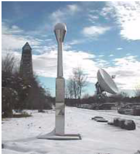
Figure 9. GPS network sites in Japan are housed in 5 meter tall stainless steel towers, as shown above. The sites are maintained by private companies under government contract; communications are provided via telephone.
