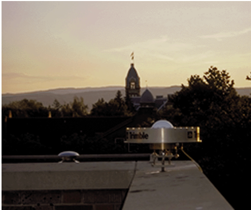
Figure 10. Standardized GPS choke ring antenna mounted on the roof of Lind Hall at Central Washington University. Similar installations are expected for universities interested only in atmospheric applications.
