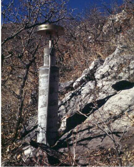
Figure 12. GPS antenna and monument established by the University of Utah for combined atmospheric and geodetic measurements, with assistance from the UNAVCO Facility.
