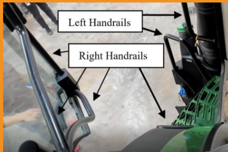
(Left) Demonstration of AG-OMS Machine learning algorithm identifying high safety risk behavior during tractor egress. (Right) Diagram of handrails on one tractor to compare with user behavior (high, medium, low safety risk) and interaction with these handles. This is important for informing future design modifications or other interventions.
