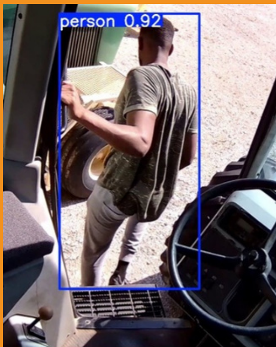
(Left) Demonstration of AG-OMS Machine learning algorithm identifying high safety risk behavior during tractor egress. (Right) Diagram of handrails on one tractor to compare with user behavior (high, medium, low safety risk) and interaction with these handles. This is important for informing future design modifications or other interventions.
