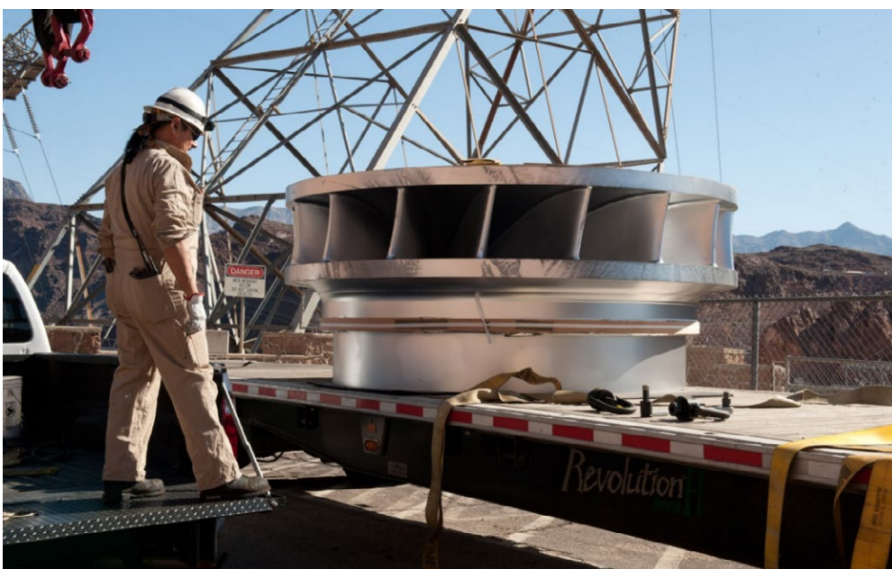
A wide-head turbine from Hoover Dam.
