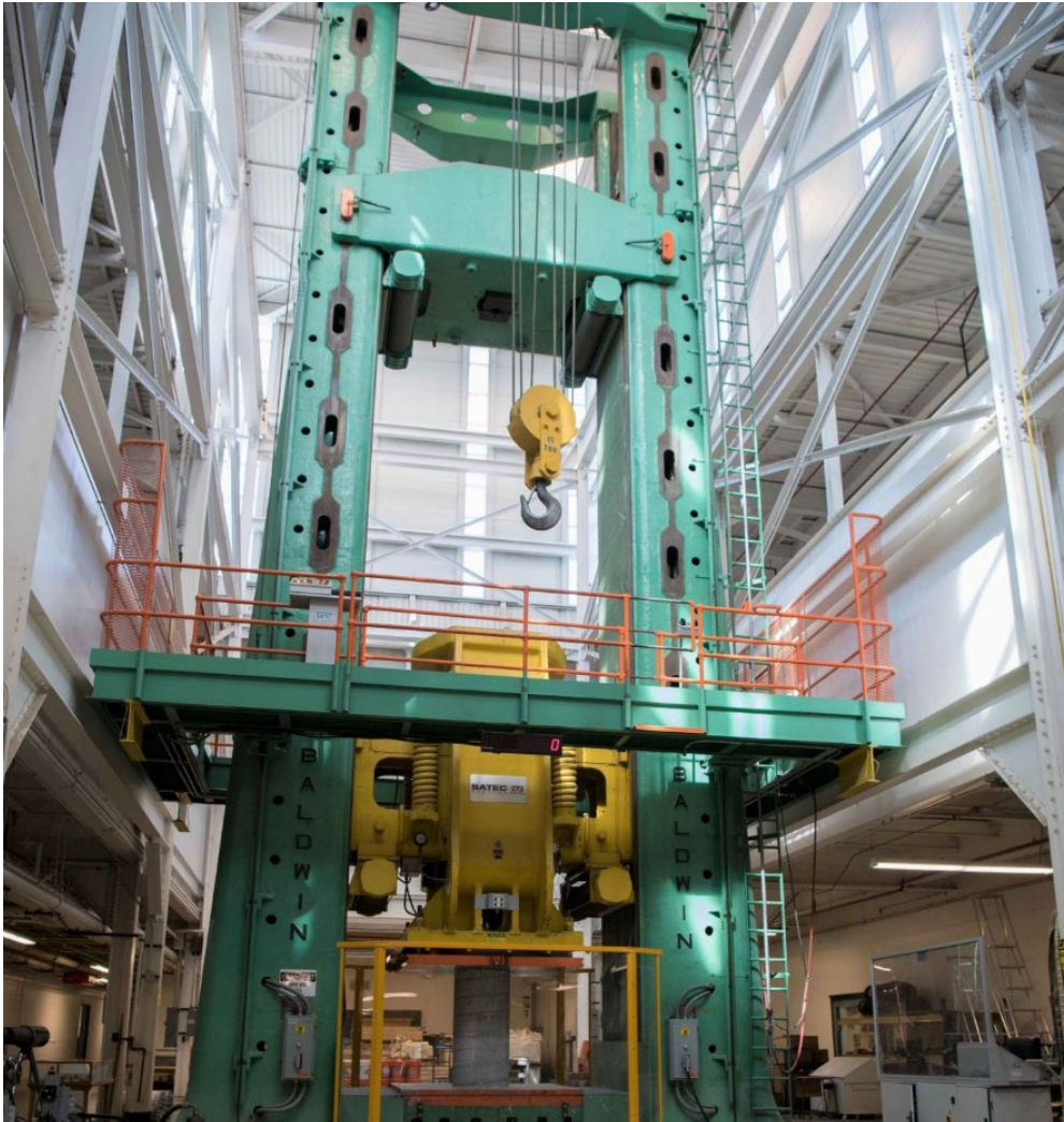
This 5-million-pound universal testing machine is located in Reclamation's Concrete and Structural Laboratory. In support of Reclamation projects, it is capable of testing the structural strength of large-size specimens, such as concrete piers.
