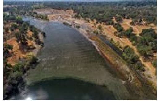
Ancil Hoffman floodplain on the lower American River. This project recreated spawning and rearing habitat by constructing new gravel beds in the river and carving a new alcove to protect juvenile fish near Ancil Hoffman Park, halfway between Folsom Dam and downtown Sacramento.
