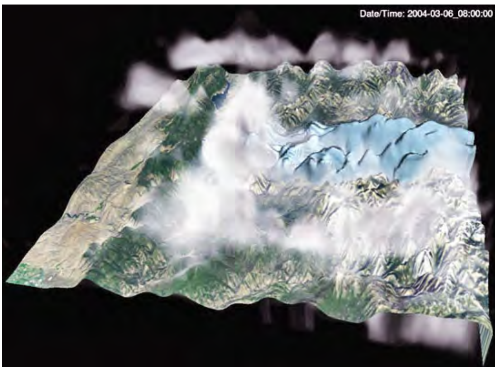
Three-dimensional rendition of the silver iodide dispersion (cyan) among a cloud field (white) over complex terrain (Xue et al. 2017).
