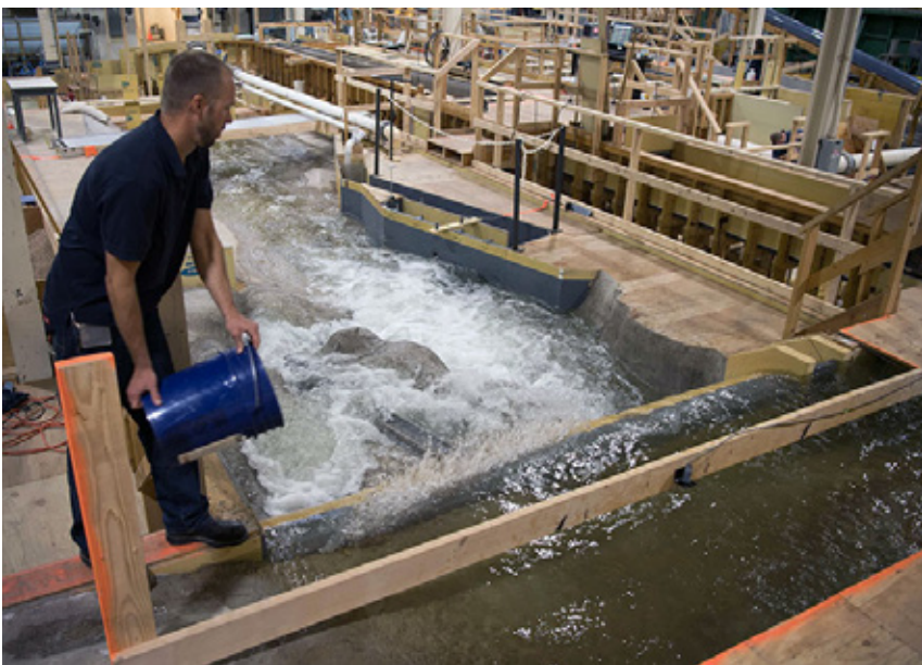
Kent Walker, a Hydraulic Engineer with Reclamation, is seen testing settlement and flow with sediment using one of the dam models.
