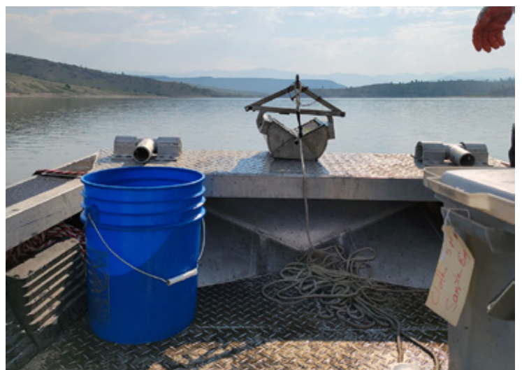
PONAR sampler used to collect surface sediment samples from the bottom of Willow Creek Reservoir. (photo courtesy of Rob Hilldale)
