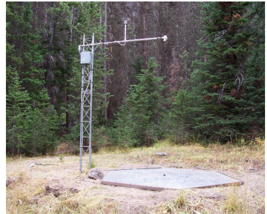
A snow depth sensor shown above a snow pillow. Photo courtesy of Natural Resources Conservation Service.
