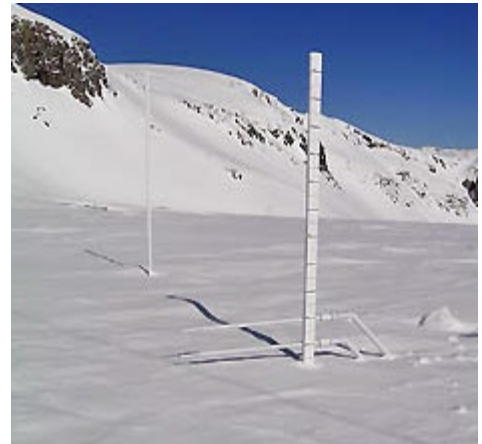
Snow temperature sensor at the Center for Snow and Avalanche Studies site in Senator Beck Basin, Colorado (Center for Snow and Avalanche Studies, used by permission).
