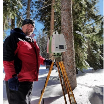
Terrestrial Laser Scanning system being set-up, Grand Mesa SnowEX. Photo courtesy of U.S. Army Corps of Engineers.
