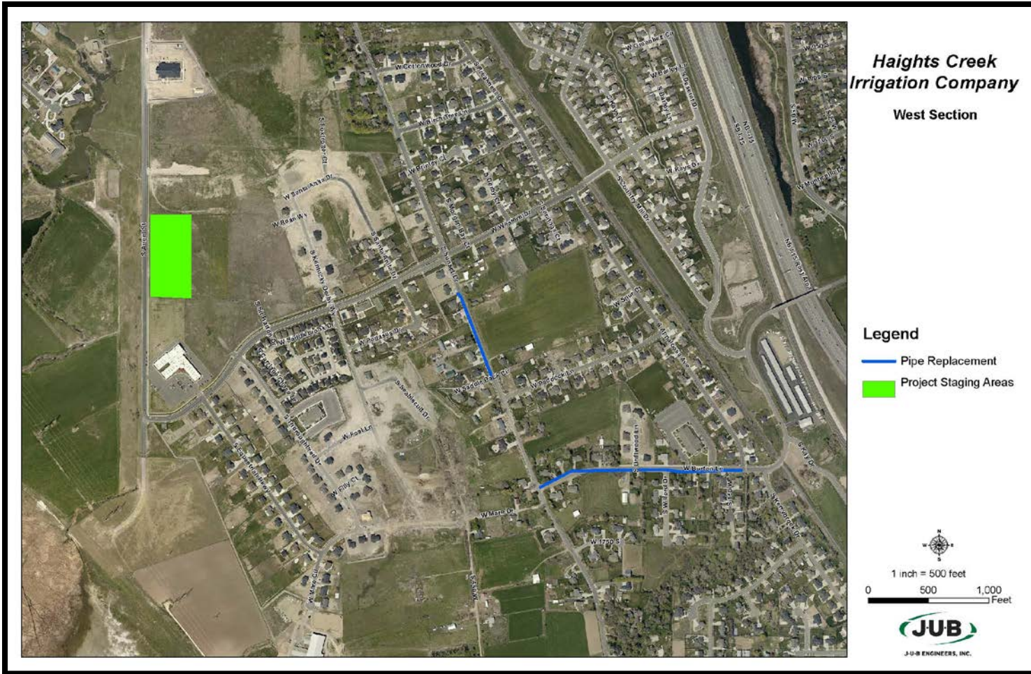
Figure 2-2 Project Alignment West
