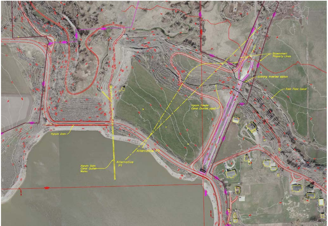
Figure 2. Drawing of all the original Action Alternatives alignments, with a backdrop of aerial imagery and topography for the Hyrum spillway.
