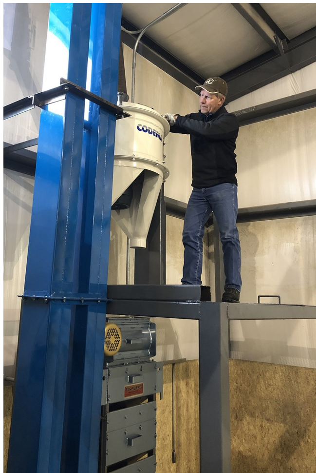
Mike Moore installs a dehuller machine at UW’s Powell Research and Extension Center. Seeds of first grains require an extra step of de-hulling prior to processing. Moore is director of the Wyoming Seed Certification Service based at the center.
